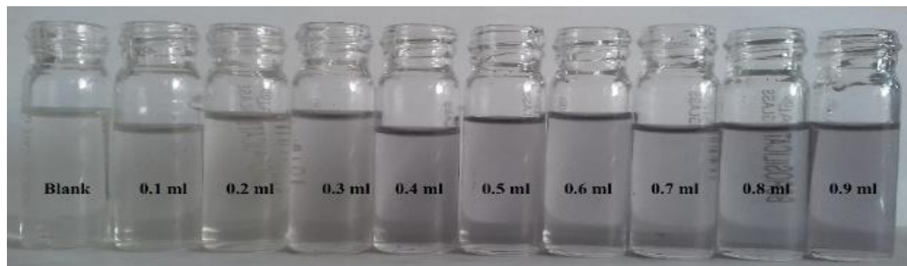
Fig. 3. Photograph of change color observed when addition of Au 3+ ions increase from 0.1 to 0.9 mL and keeping the concentration of 3 constant.
