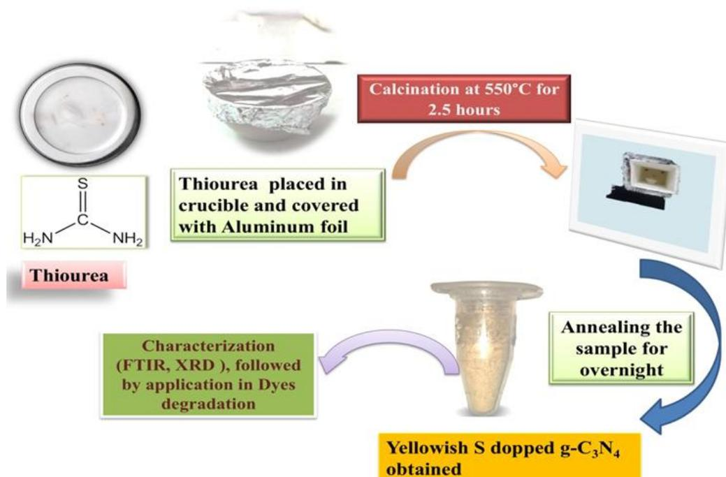
**Fig. 1.** Schematic illustration of the thermal polymerization synthesis process for sulfur-doped graphitic carbon nitride (S-g-C<sub>3</sub>N<sub>4</sub>) using thiourea as precursor. The process involves controlled pyrolysis at 550 °C followed by ethanol washing and drying to obtain the final photocatalyst.
